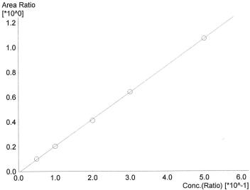
Name : Ethanol Detector Name: FID1 Function : f(x)=2.16010\*x-0.0123065 (R^2 value= 0.9997823) FitType: Linear ZeroThrough: Not Through
